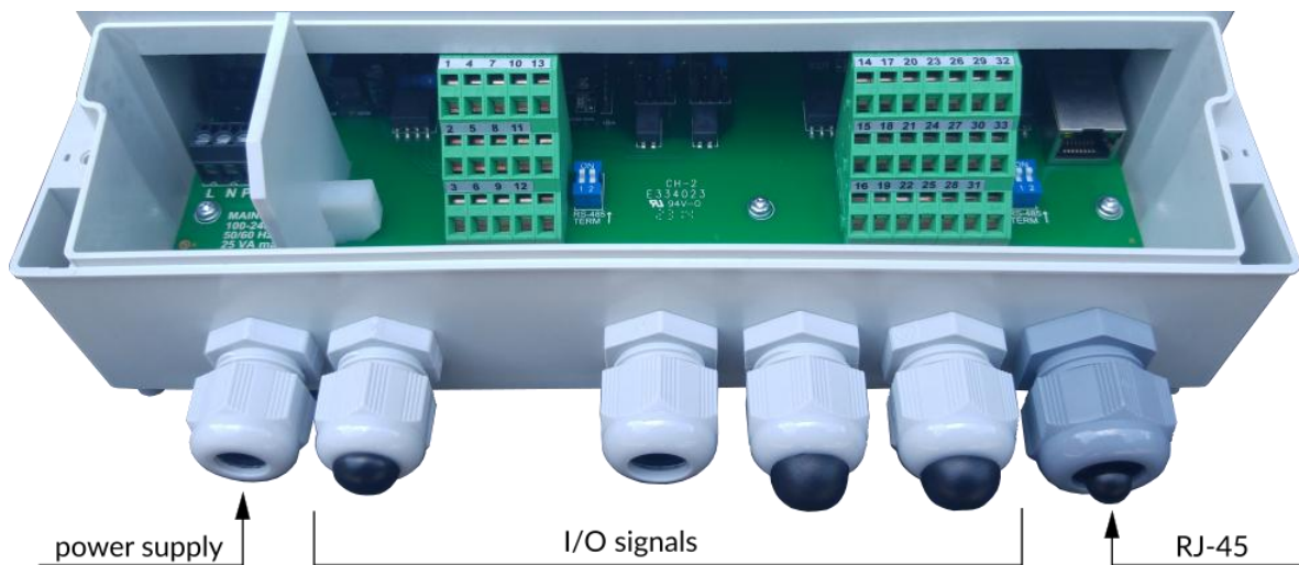
Pin type spring terminal block in MPI-DN recorder
