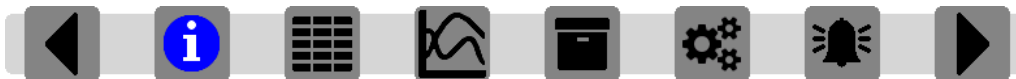
Fig. 7.3 Touching the screen at the height of the title bar shows up menu bar.
